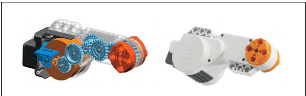
Figures 1. 4: Structure of NXT Servomotor [1]
