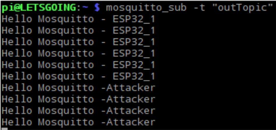
A terminal window on a Raspberry Pi (pi@LETSGOING) showing the execution of the command 'mosquitto\_sub -t "outTopic"'. The output shows a sequence of messages: six 'Hello Mosquitto - ESP32\_1' messages, followed by three 'Hello Mosquitto -Attacker' messages. This demonstrates the successful manipulation of the received MQTT messages.
